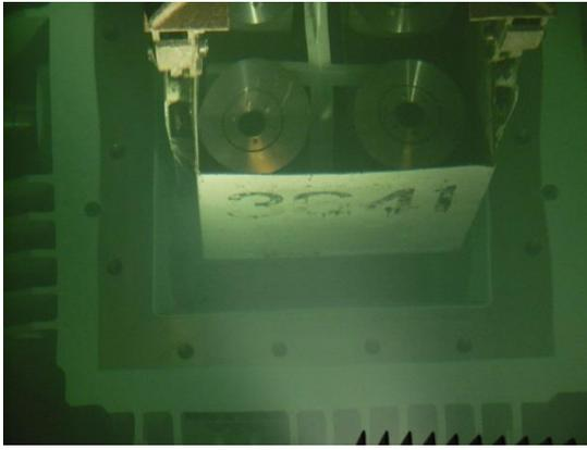
ION SIV cartridges are loaded into a transport flask
