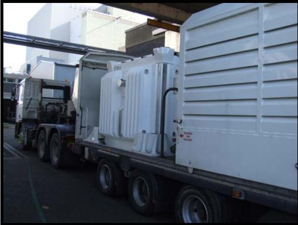
Fuel flask loaded onto flask transporter
